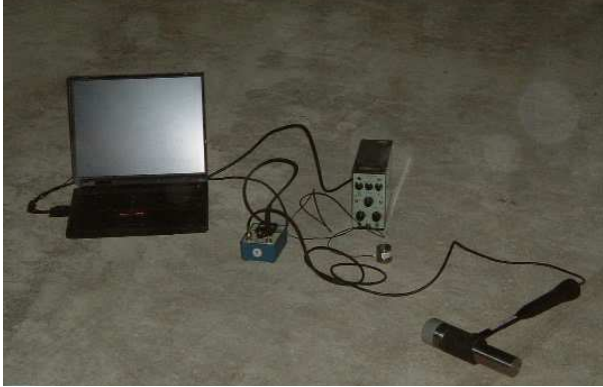
Fig. 7. Setup of the instrumented hammer test.
