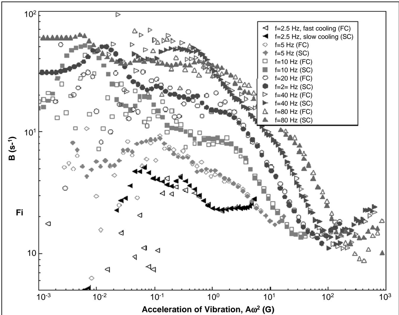
Figure 2. Damping Prediction on Parallel Computers as a Function of Acceleration (g)
