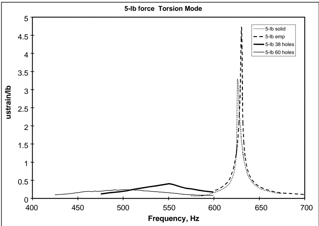
Figure 3. Plate Response to Sine Inputs of Solid, 38 and Holes Filled Configurations
