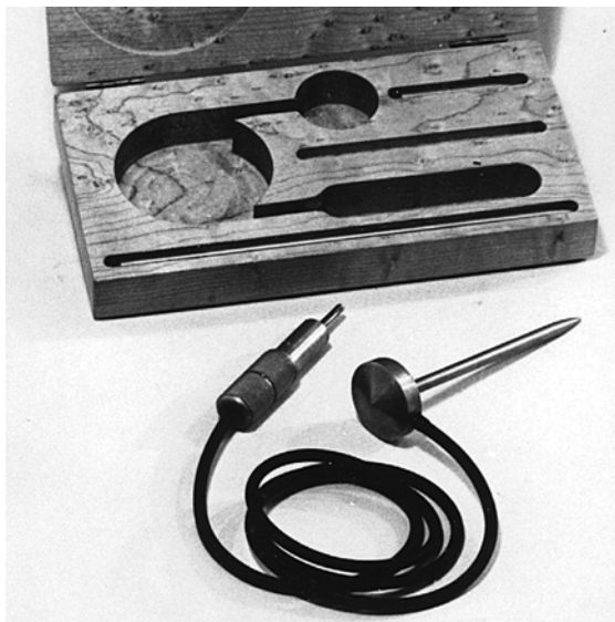
Figure 2. Configuration of First Manufactured Accelerometer (B&K)
