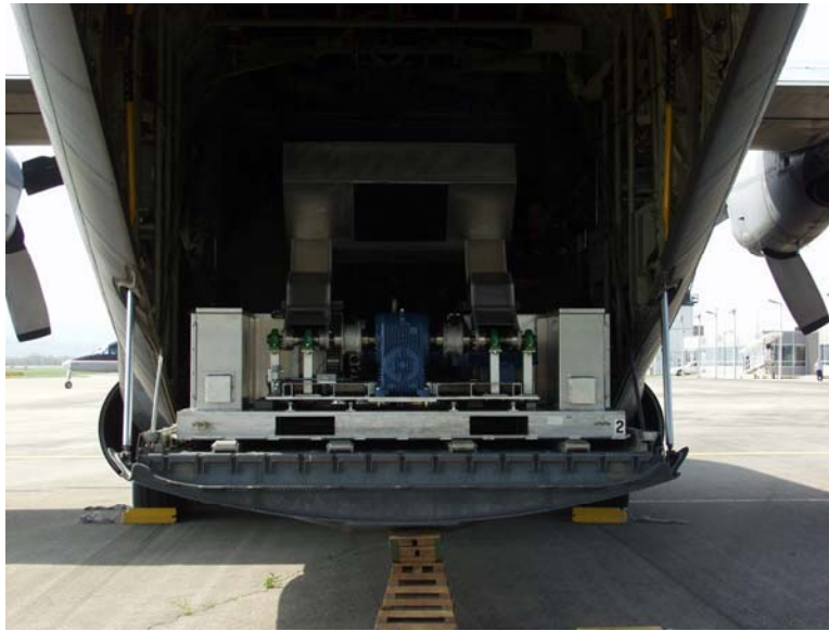
Figure 2 – Sensor pallet system in stow position in a C-130 aircraft.
