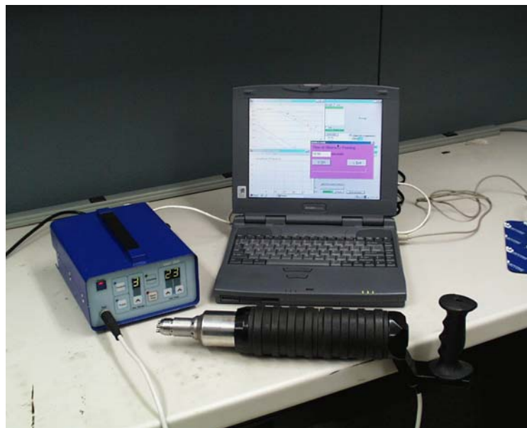
Figure 6. Computerized Complex for Ultrasonic Peening of parts and welded elements
