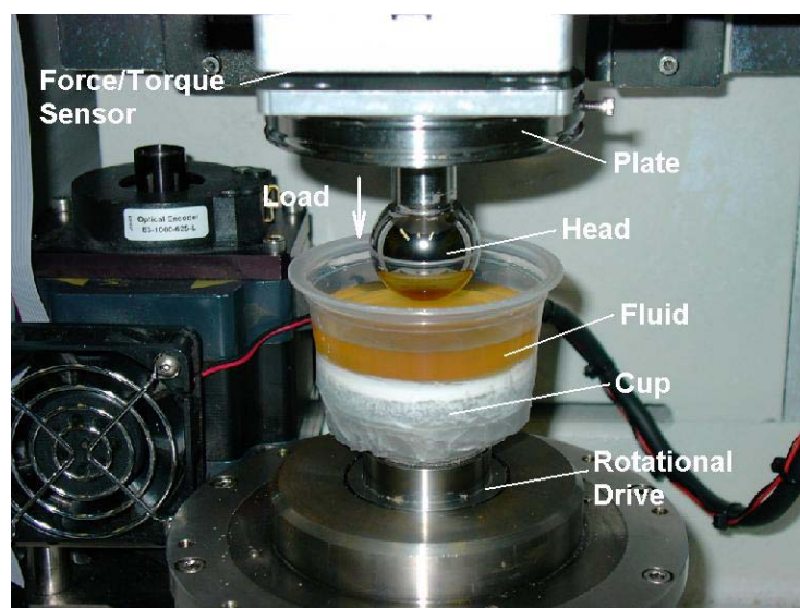
Figure 7. Hip Joint Test Setup
